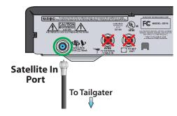
**b.** Connect the other end of the coaxial cable to the coaxial port on the Tailgater.
